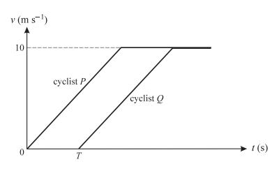
The diagram shows the velocity-time graphs for the motion of two cyclists P and Q, who travel in the same direction along a straight path. Both cyclists start from rest at the same point O and both accelerate at  $2 \text{ m s}^{-2}$  up to a speed of  $10 \text{ m s}^{-1}$ . Both then continue at a constant speed of  $10 \text{ m s}^{-1}$ . Q starts his journey T seconds after P.
