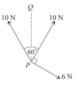
Three coplanar forces of magnitudes 10 N, 10 N and 6 N act at a point *P* in the directions shown in the diagram. *PQ* is the bisector of the angle between the two forces of magnitude 10 N.
